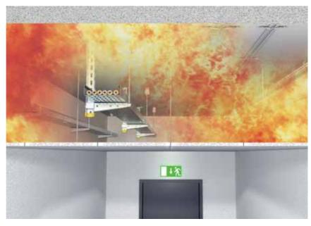
Escape route installation system above a suspended fire protection ceiling
