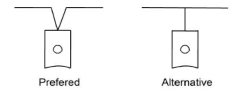
Figure 3a. Connection to Modules
