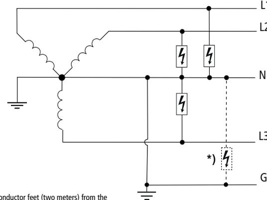
\*) Note: If the DEHNbloc DB M 1 320 (FM), (secondary surge arrester) are installed more than six conductor feet (two meters) from the neutral to ground bond point (usually service entrance), then an additional DEHNbloc should be installed between neutral and ground.
