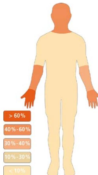
The hand and forearm region is particularly at risk of being burnt by arc faults whilst working at electrical installations.
