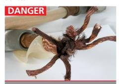
Approx. 30 year old set with reduction of area due to copper corrosion
