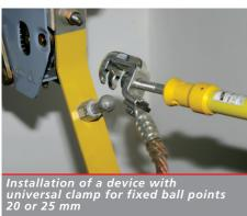
The most important rule of the five safety rules is earthing and short-circuiting. This secures isolation of the system from power supply while works are carried out even in the case of interference voltages, surges of atmospheric origin or accidental re-start. However, this safety measure is also only as good as the device used.
