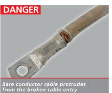
Any damage of the cable sheath or protrusion of bare conductors presents severe damage which means that the device cannot be used anymore.
