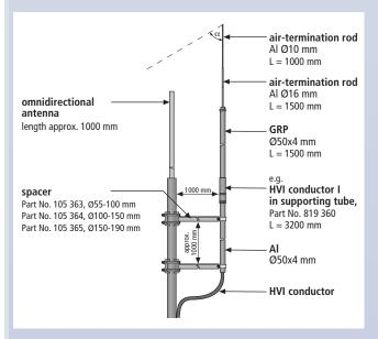
Figure 2: Exemplary design for an omnidirectional antenna, length 3000 mm
