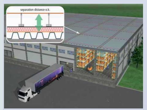
Non-compliance with the separation distance can lead to sparkover from the external lightning protection system conductors to electrical and metal installations inside of the building or
