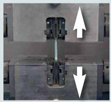
Figure 7: Tensile testing of conductors
