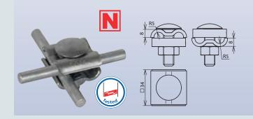
connection of round conductors for cross connections, T connections, parallel connections and double conductor connections
