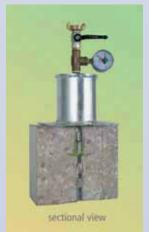
**Figure 2:**Set-up with terminal for the pressure-water test
