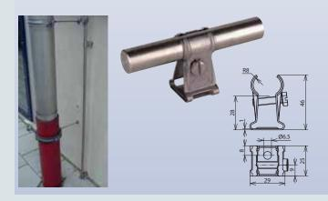
Rod holder for wall mounting with fixing screw M6, fixed conductor leading
