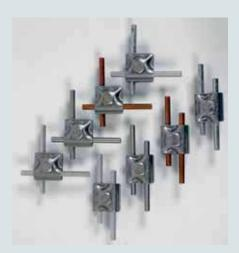
Figure 4: Test combinations for MV clamps (parallel and cross arrangement)
