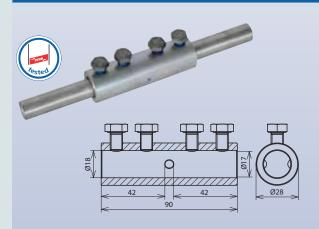
Connecting sleeve with tongues (stop) for jointing air-termination rods to greater lengths (transport length)
