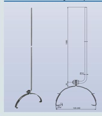
Air-termination rod for protecting solar thermal modules or photo-voltaic generators, or other superstructures on gable roofs
