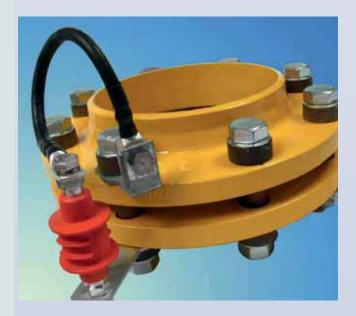
The Ex isolating spark gaps of the EXFS 100 / EXFS 100 KU product family are used when conductive installation components situated in explosion-hazard areas cannot be connected directly with each other. The spark gaps with low sparkover voltage are especially efficient for isolated installation components with little insulation resistance.
