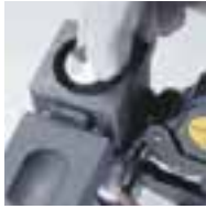
Step 2 Close mould and drop metal disk in place
