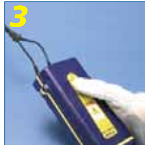
3 Press and hold control unit switch and wait for the ignition
