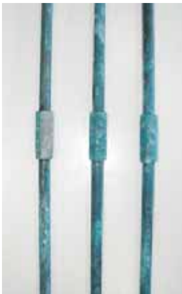
Specimens after salt spray tests
