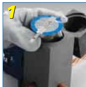
1 Insert CADWELD PLUS package into mould
