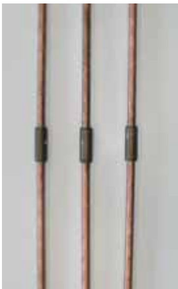
Specimens before salt spray tests
