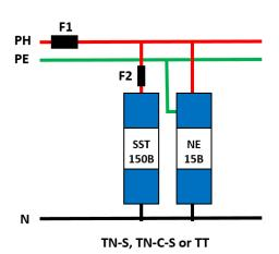
Note: For 100 kA and above, connect the Ph1 to one of the SST150B modules only.
