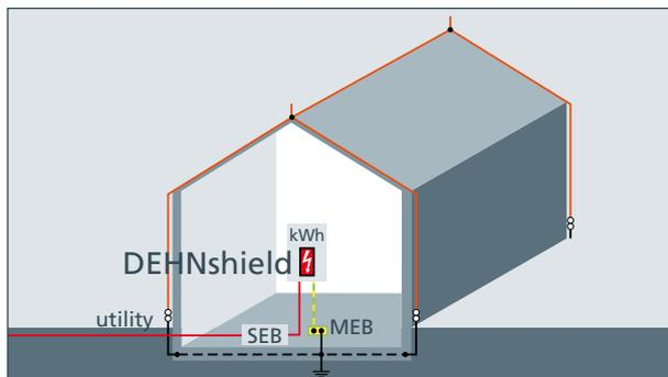
For buildings with external lightning protection system and a compact and simply equipped electrical installation with low technical requirements.
