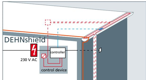
For use with gutter heating systems to protect the electrical installation from incoming lightning currents.
