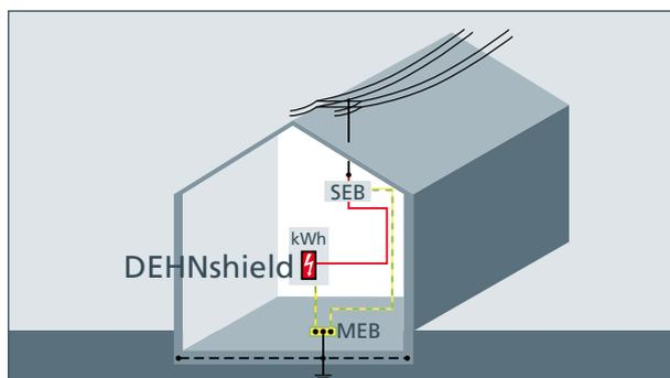
For buildings without external lightning protection system where power is supplied through an overhead line.
