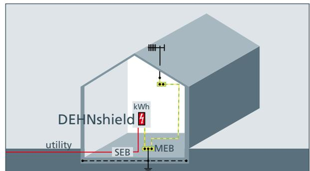
For buildings without external lightning protection system on which roof superstructures, for example antennas, are installed.
