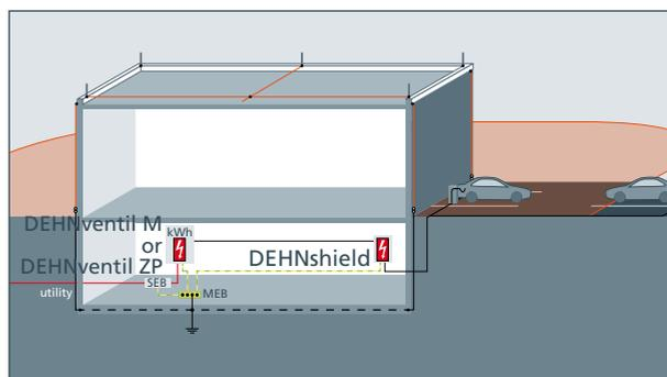
For connecting outdoor electrical loads (LPZ 0<sub>A</sub>) to the power supply system in the main building, for example, exterior lighting or charging station for electric vehicles.
