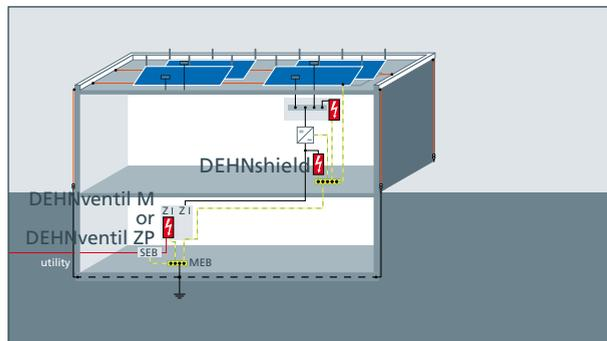
Protection of inverters which are more than ten metres away from a main distribution panel, if the separation distance from the external lightning protection system is not kept.
