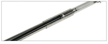
**Step 2:** The head piece for the installation of HVI®power is fixed using a locking screw on the side of the supporting tube. The position of the screw shows whether the HVI®power conductor is installed correctly.
