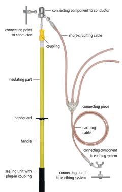
Safe insulation of the operating staff will be achieved by the correct application of insulating means. Usually not the insulating characteristics are decisive for the length of an earthing stick but rather the necessity to provide a sufficient distance from unearthed parts of the electrical system in case of earthing and short-circuiting.
