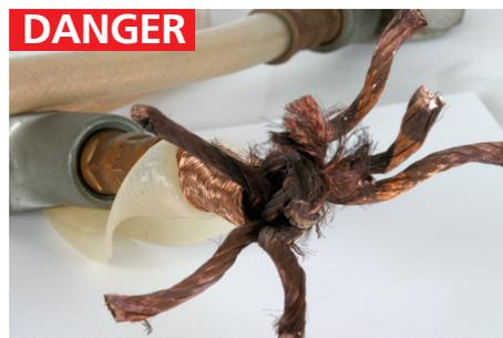
Approx. 30 year old set with reduction of area due to copper corrosion
