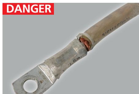
Bare conductor cable protrudes from the broken cable entry
