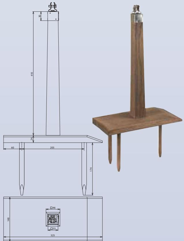
**Support St/tZn for Use at Eaves**for guying the conductors at eaves
