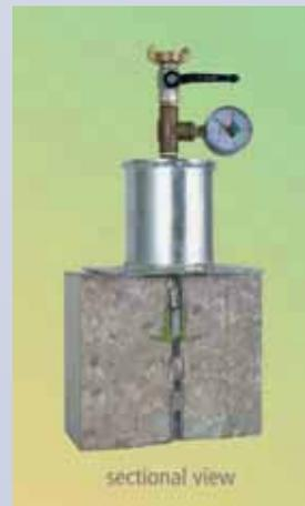
Figure 2: Set-up with terminal for the pressure-water test
