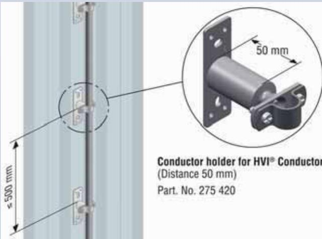
Schematic illustration – installation in Ex zones 1 or 2 and 21 or 22 at a metal facade
