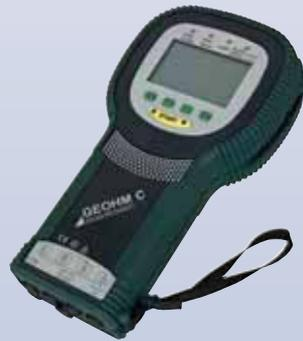
Earthing resistance meter for measuring of earthing resistance and soil resistivity. The device provides automatic measuring range selection for checking the earthing resistance of sensors and auxiliary earth-electrodes.
