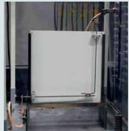
Figure 5: Specimen fixed on insulating plate (MV clamp) for a test in the impulse current laboratory
