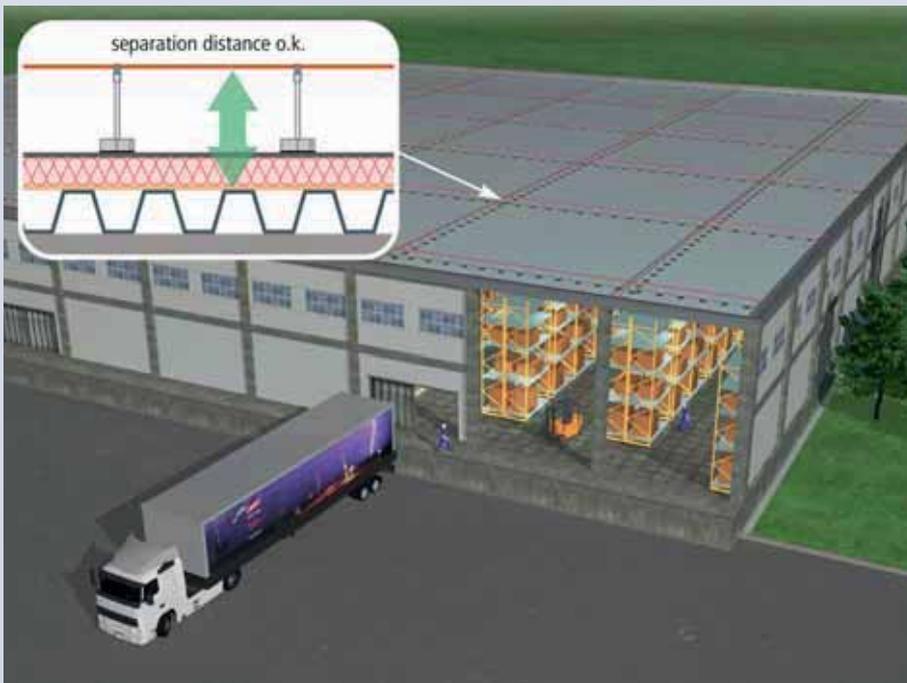
Non-compliance with the separation distance can lead to sparkover from the external lightning protection system conductors to electrical and metal installations inside of the building or structure.
