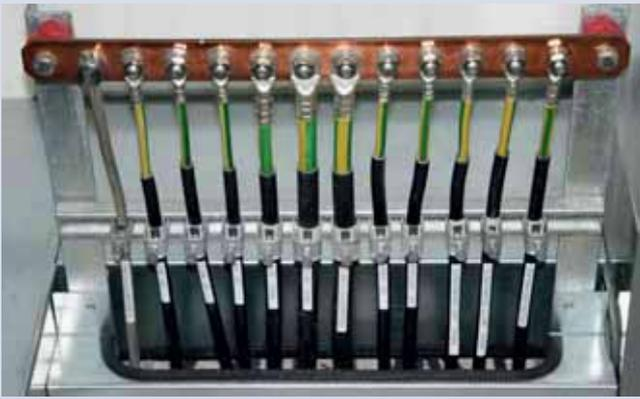
Equipotential busbars for the protective and functional equipotential bonding and lightning equipotential bonding according to EN 62305-3 also for use in potentially explosive atmospheres (screws are locked to prevent accidental loosening)
